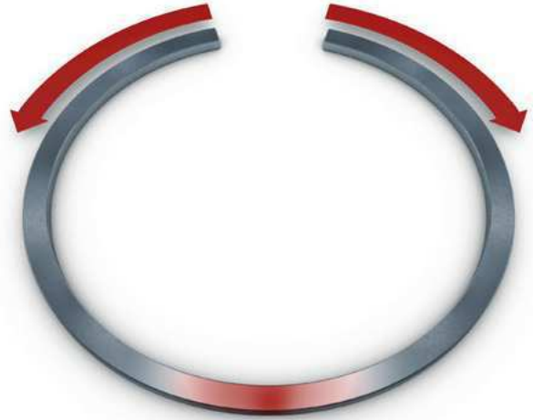
Fig. 1: Excessive spreading of the piston ring
