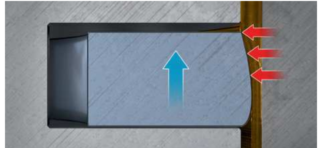
Fig. 4: High floating during the upwards movement
