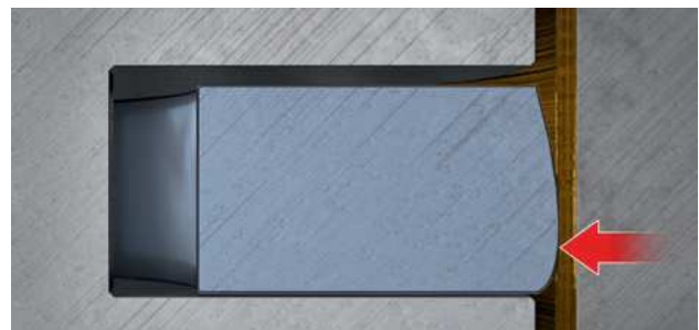
Fig. 3: Asymmetrically crowned piston ring sliding surface
