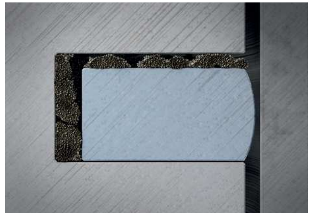
Fig. 1: Dirt deposit in the ring groove
