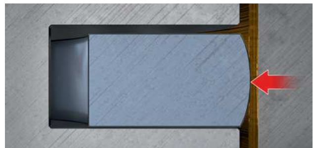
Fig. 2: Symmetrically crowned piston ring sliding surface
