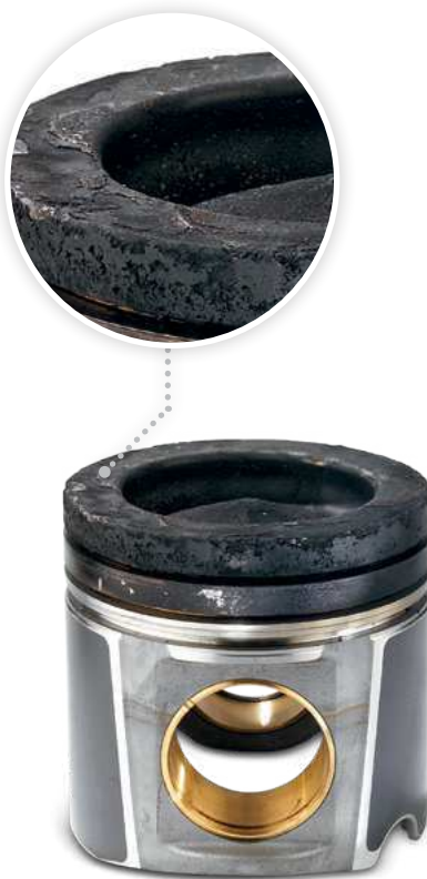
Fig. 3: Carbon layer on the top land
