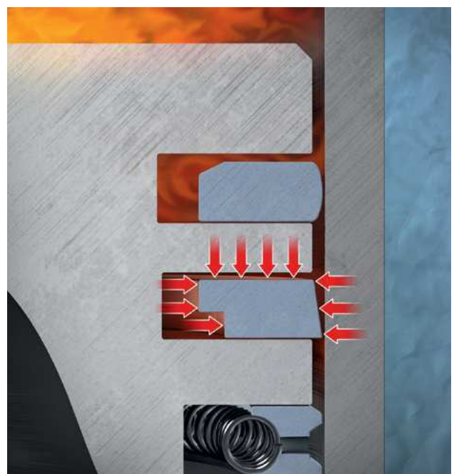
Gas pressure on the taper faced ring
