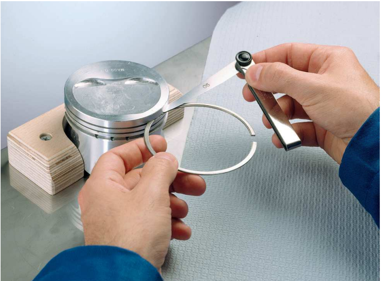
Fig. 1: Measuring the ring height clearance
