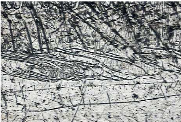
Fig. 4 and 5: Examples of roller marks on the top ring side
