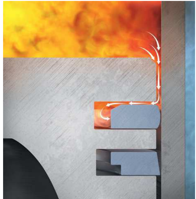
Sealing against combustion gases
