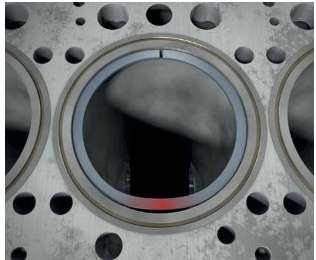
Fig. 2: Formation of crescent-shaped gaps due to excessive spreading
