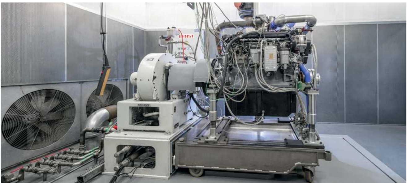
Running-in and wear tests on the engine test rig
