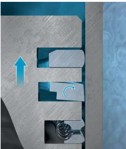
Fig. 5: Without combustion pressure
